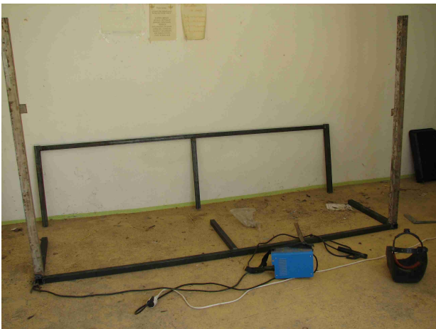
Tubes acier soudés constituant le support
